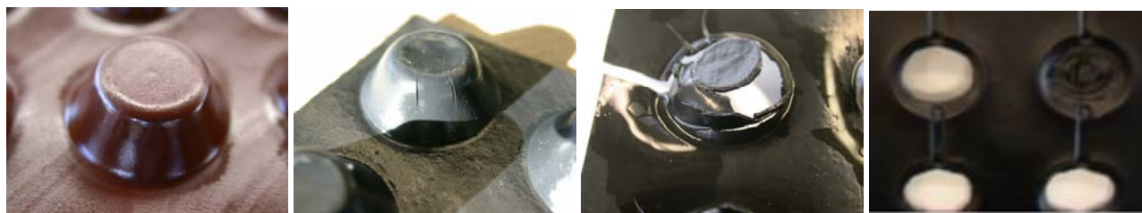
(a) No failure (b) Cracking (c) Severe cracking (d) Severe cracking
