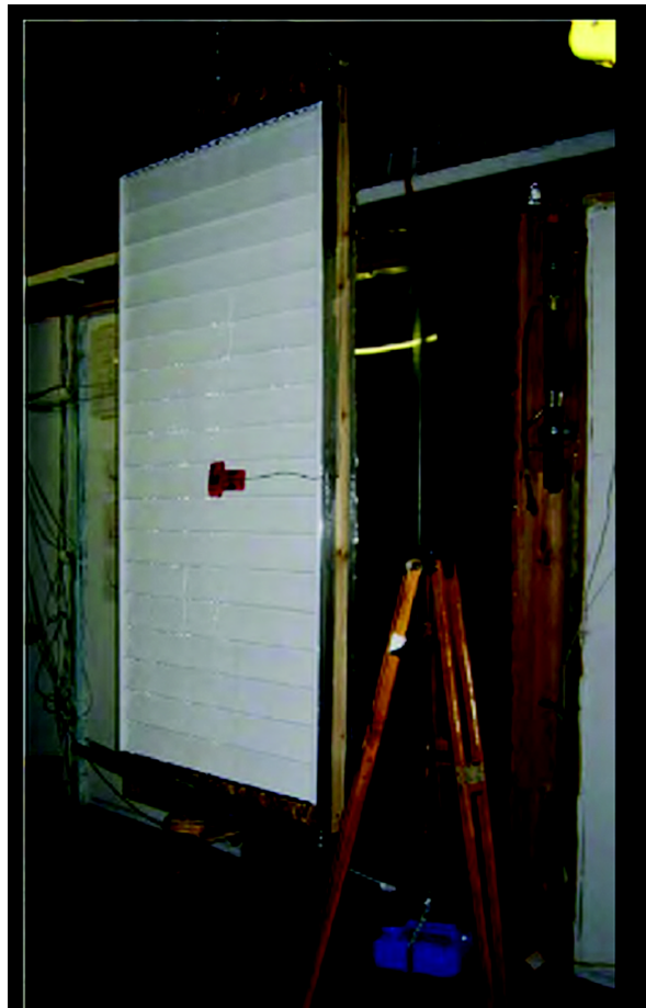
Figure 5 Drainage testing of embossed PE weather resistive barrier system (Straube et al. 2005).
